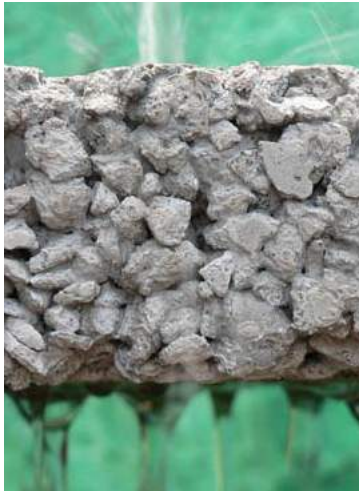
FIGURE 2 Impervious v. Pervious Pavements Photograph on the left shows a section through a typical impervious pavement. The section on the right shows a pervious pavement that is designed to allow percolation or infiltration of stormwater through the surface into the soil below where the water is naturally filtered and pollutants are removed.
