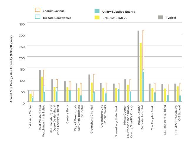
By comparing the gray bars (typical energy use) with the blue bars (utility-supplied energy), one sees significant energy savings across the board. The dashed orange bars indicate overall energy savings, which reflect the rigorous design and construction required for each one.
